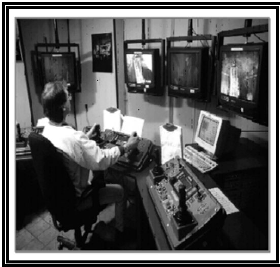
Control room for operating remote mining equipment (photo courtesy of INCO - Mining Automation Program).
