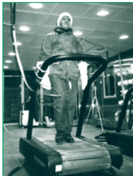
Volunteers equipped with heat-flow sensors and thermocouples participated in four 90-minute tests at different temperatures and wind speeds inside a refrigerated wind tunnel.
