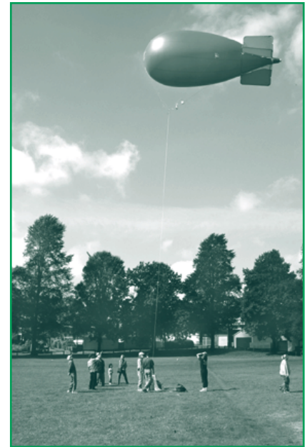
A tethered weather balloon at the Slocan site in Burnaby. The balloon was released to a height of about one kilometre, and then winched back down to provide a vertical profile of ozone and meteorological parameters, including wind speed and direction, humidity and temperature.
