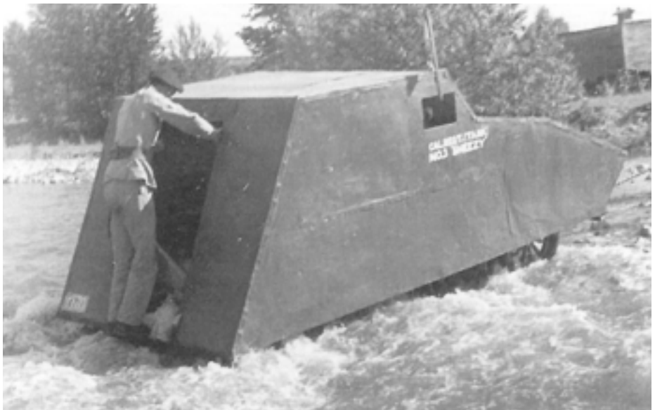
Innovation at work. As in Germany, Canada conducted armoured training and trials with mock tanks, albeit with spectacularly different results. Here one such vehicle built using a Model A Ford car, is used by the King’s Own Calgary Regiment to practice “amphibious” landings. (Courtesy KOCR Museum)
