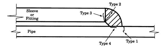
Type 1- Toe crack
