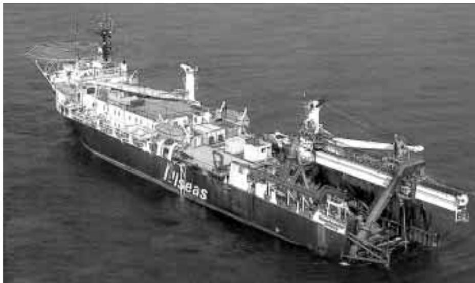
Figure 4. Photograph of a Typical Pipe-Lay Barge
