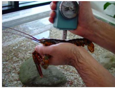
Figure 2. Durometer reading positions on the cephalothorax (a) anterodorsal region A and (b) dorsolateral region B, as well as (c) the measurement of the lobster carapace length with an electronic caliper.
