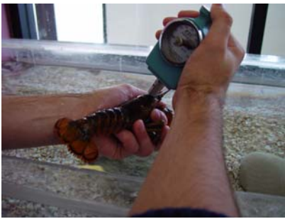
Figure 2. Durometer reading positions on the cephalothorax (a) anterodorsal region A and (b) dorsolateral region B, as well as (c) the measurement of the lobster carapace length with an electronic caliper.
