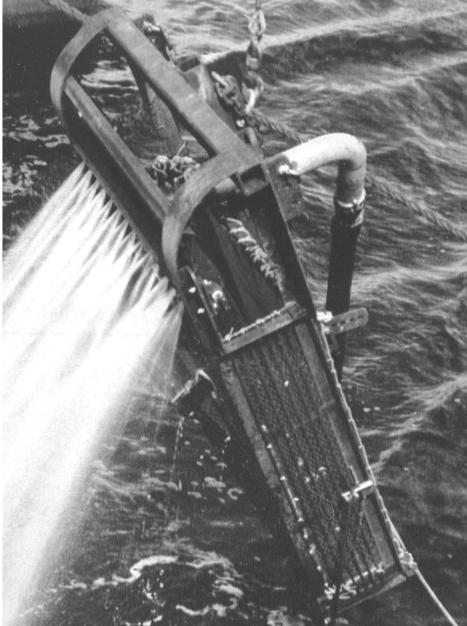
Figure 2. New England style hydraulic clam dredge (Lambert and Goudreau 1996)
