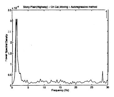
Fig. 6 Vibration: Power spectra of vibration on police officers in police vehicle during municipal policing
