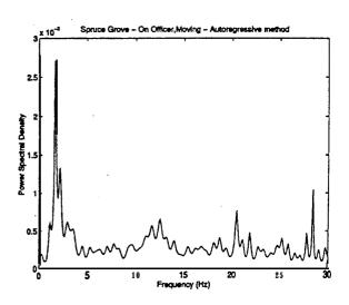
Fig. 7 Vibration: Power spectra of vibration on police officers in police vehicle during rural policing
