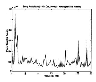
Fig. 5 Vibration: Power spectra of police vehicle during highway patrol
