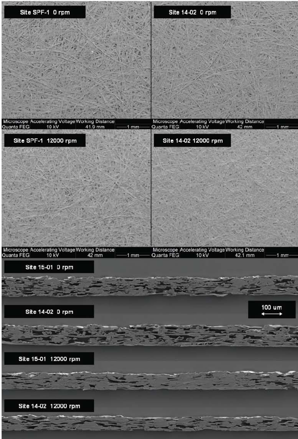
Figure 24. Cross-section and surface images of selected kraft handsheets before and after PFI mill refining.
