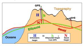
For Canada, the geoid heights can be obtained from the Canadian Gravimetric Geoid model 2005 (CGG2005).
