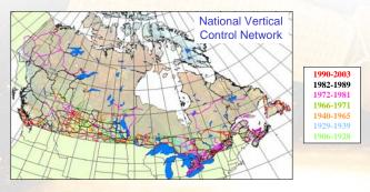
The Canadian Geodetic Vertical Datum of 1928 (CGVD28) was realized in 1928 by doing a national scale adjustment of all levelling. The CGVD28 was and is still to this day the official reference surface for heights in Canada. However it is not error-free:
