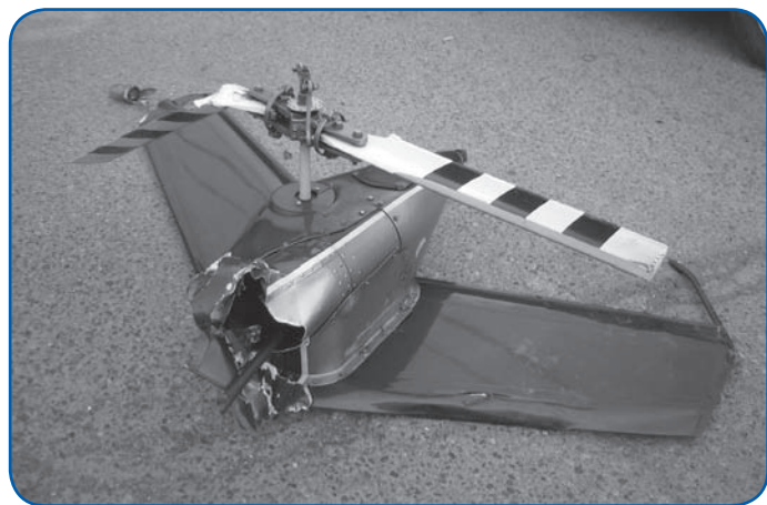
Tail rotor unit shown at the accident scene. The main and tail rotor blades were relatively undamaged.
