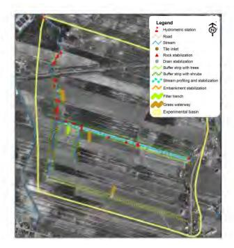
Figure 15a: Runoff and erosion control structures in the Fourchette intervention micro-watershed
