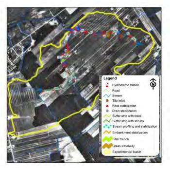
Figure 15b: Runoff and erosion control structures in the Bras d'Henri intervention micro-watershed
