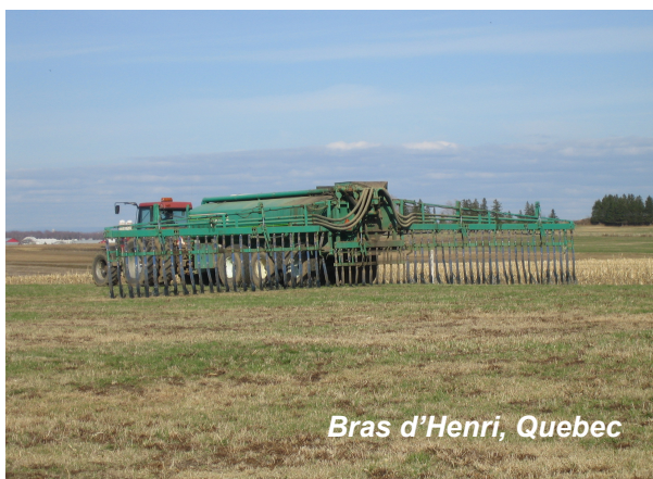
Figure 4: The hog slurry management BMP uses spreaders adapted with trailing hoses in order to reduce nitrogen losses to the atmosphere.
