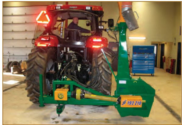
The willow harvester hooked up to a tractor. Photo: Chris Pharo
