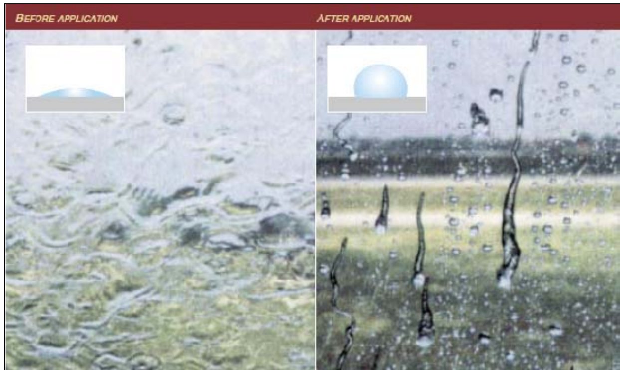
Photo 2. Effect of rain repellent on water droplet/windshield contact angle. 6
