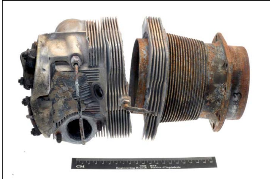
Figure 1. Number 3 cylinder after removal from the engine
