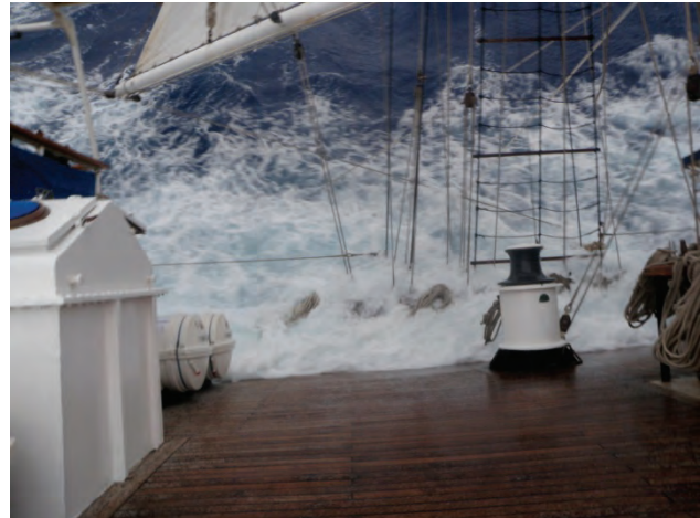
Photo 5. Port rail immersed at 41°
