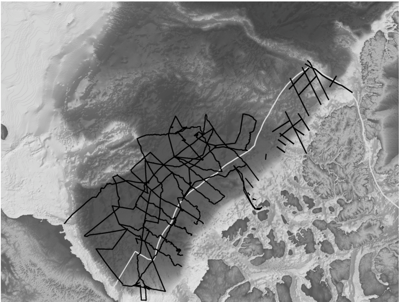
Figure 8 Overview of seismic and key bathymetry data collected over the period 2007–10. A total of over 13,500 km of seismic and over 18,000 km of bathymetry data have tripled our data holdings in the Arctic.
