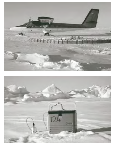
Figure 4 Image of the seismic recorders used in the LORITA and ARTA experiments. About 150 recorders were put on the ice, 1–2 km apart and this configuration was used to record crustal velocities. Photo: R. Jackson, GSC.
