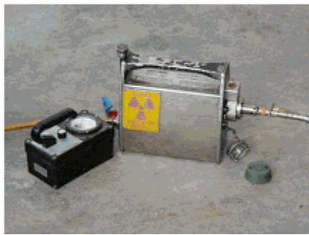
Image #5: Industrial radiography "camera" which contains the radioactive sealed source
