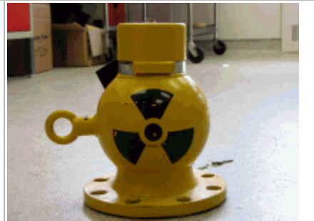
Image #7: Industrial fixed gauge
