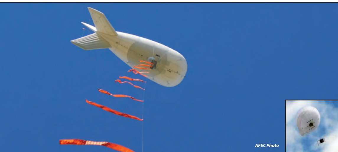
The aerostats employed for DIRE '10. The smaller lifts 16 kilograms (kg), the larger 91 kg.
