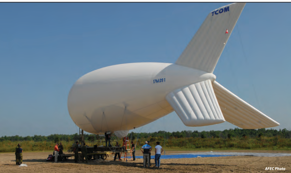
The 17-metre aerostat when docked can survive 140 km/h winds (100 km/h in flight).
