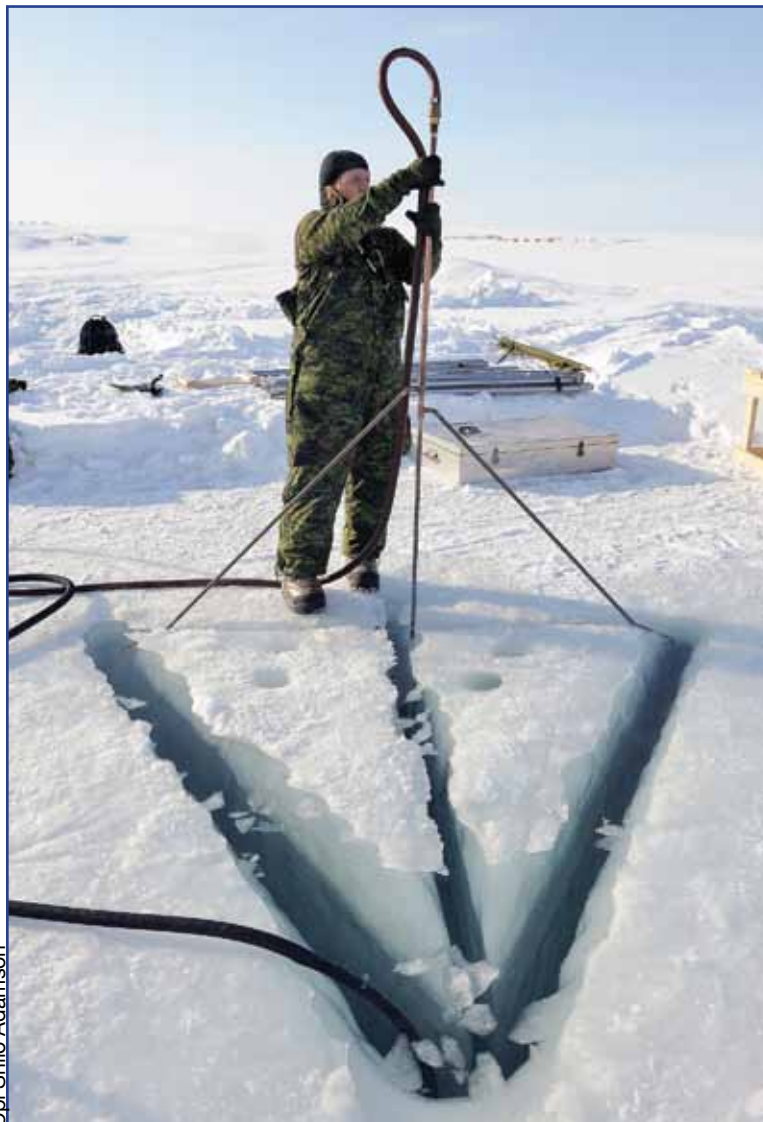
Col Shilo Adamson Master Seaman Marie Martel, a member of the Port Inspection Dive Team, adjusts the hot water intake hose as she operates the hot water saw, a device designed to cut through ice, during Operation NUNALIVUT 10.
