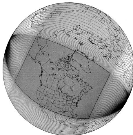
Figure 8-1 The variable-resolution horizontal grid of the operational regional configuration of the GEM model, with a uniform horizontal grid-spacing of 0.1375^\circ ( \sim 15 km) over the central window.
