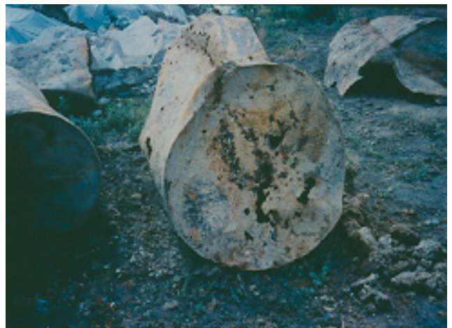
Figure 2. Exhumed leaking underground storage tanks. Photo by: D.W. Alley
