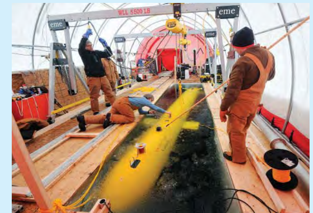
The autonomous underwater vehicle (AUV) Yamoria is a one-of-a-kind product: a remotely-controlled research submarine built to withstand the extreme pressure and cold of the Arctic undersea environment. The result of a scientific partnership between Natural Resources Canada, Defence Research and Development Canada and Fisheries and Oceans Canada and built by International Submarine Engineering Ltd. (ISE) of Port Coquitlam, B.C., Yamoria is seven metres long, 2,000 kg in weight, cylindrical in shape and powered by lithium-ion batteries that can be recharged under water. Yamoria is named for an ancient great traveler and lawmaker of the Dene people.
