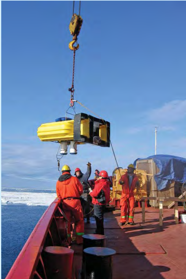
One of the moorings to measure sea ice transport in Barrow Strait is deployed from the CCGS DesGroseilliers .
