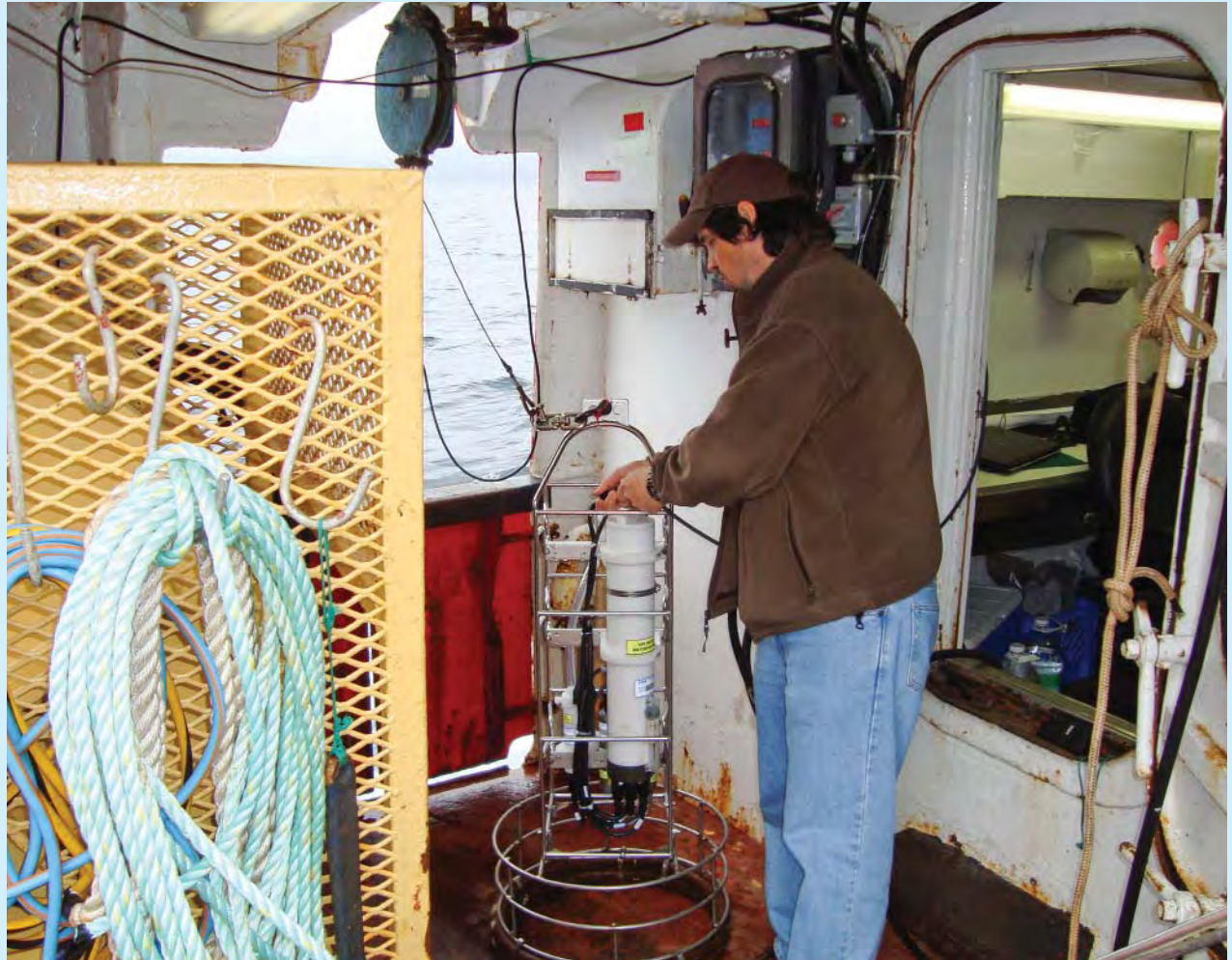
A conductivity, temperature, depth (CTD) instrument being prepared for deployment.
