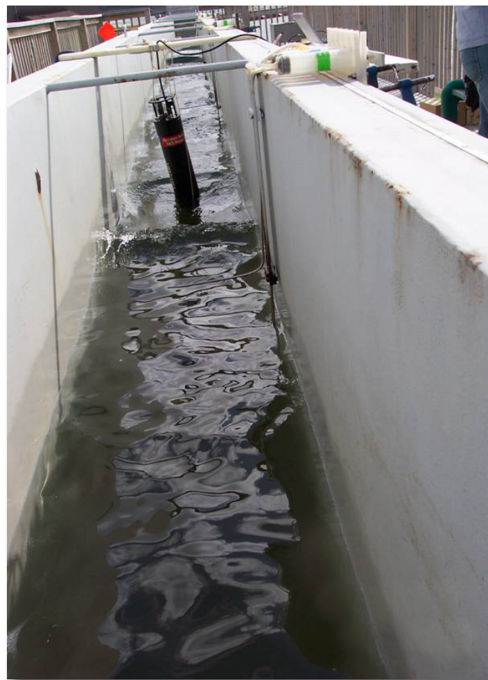
Wave tank at Bedford Institute of Oceanography used for oil dispersant studies.
