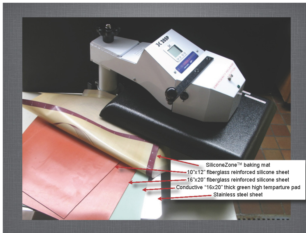
Fig. 6. DK20SP 16X20 Automatic Digital Swinger (Scale Press) and the layering order of the silicone pads and stainless sheet used for pressing scales.
