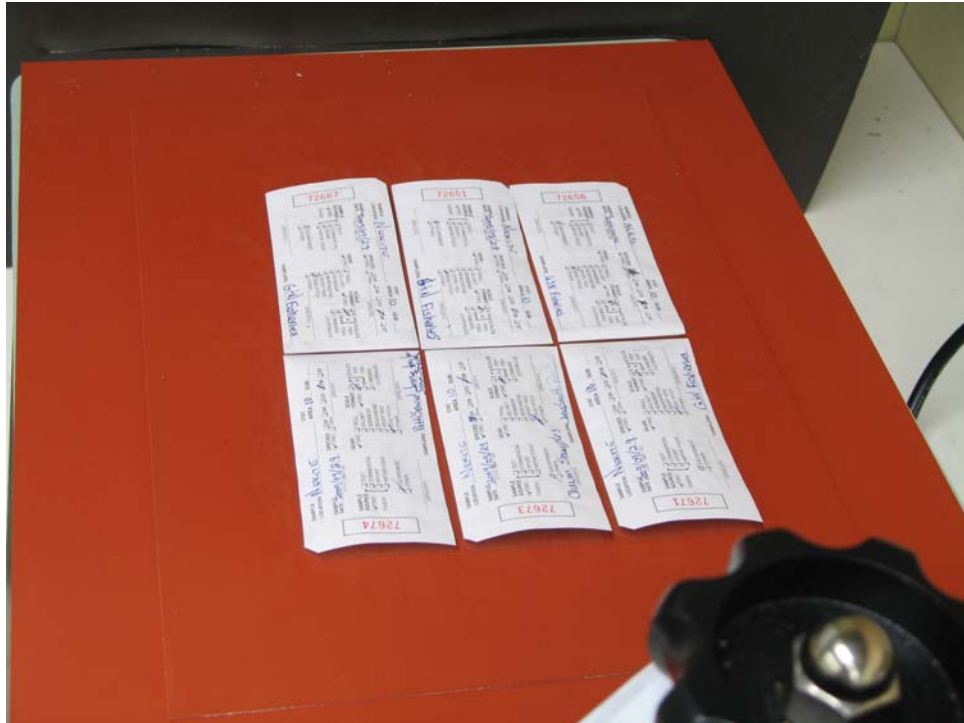
Fig. 7. Scale card placement on 10"X12" 0.062" thick fibreglass reinforced silicone sheet.
