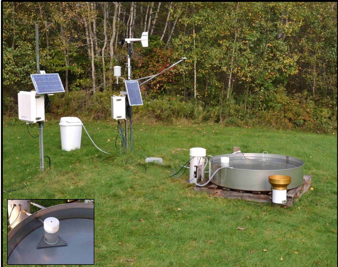
Figure 9. Installation of the prototype automatic evaporation pan for testing in the field. Figure inset shows the protective casing over the overflow apparatus.
