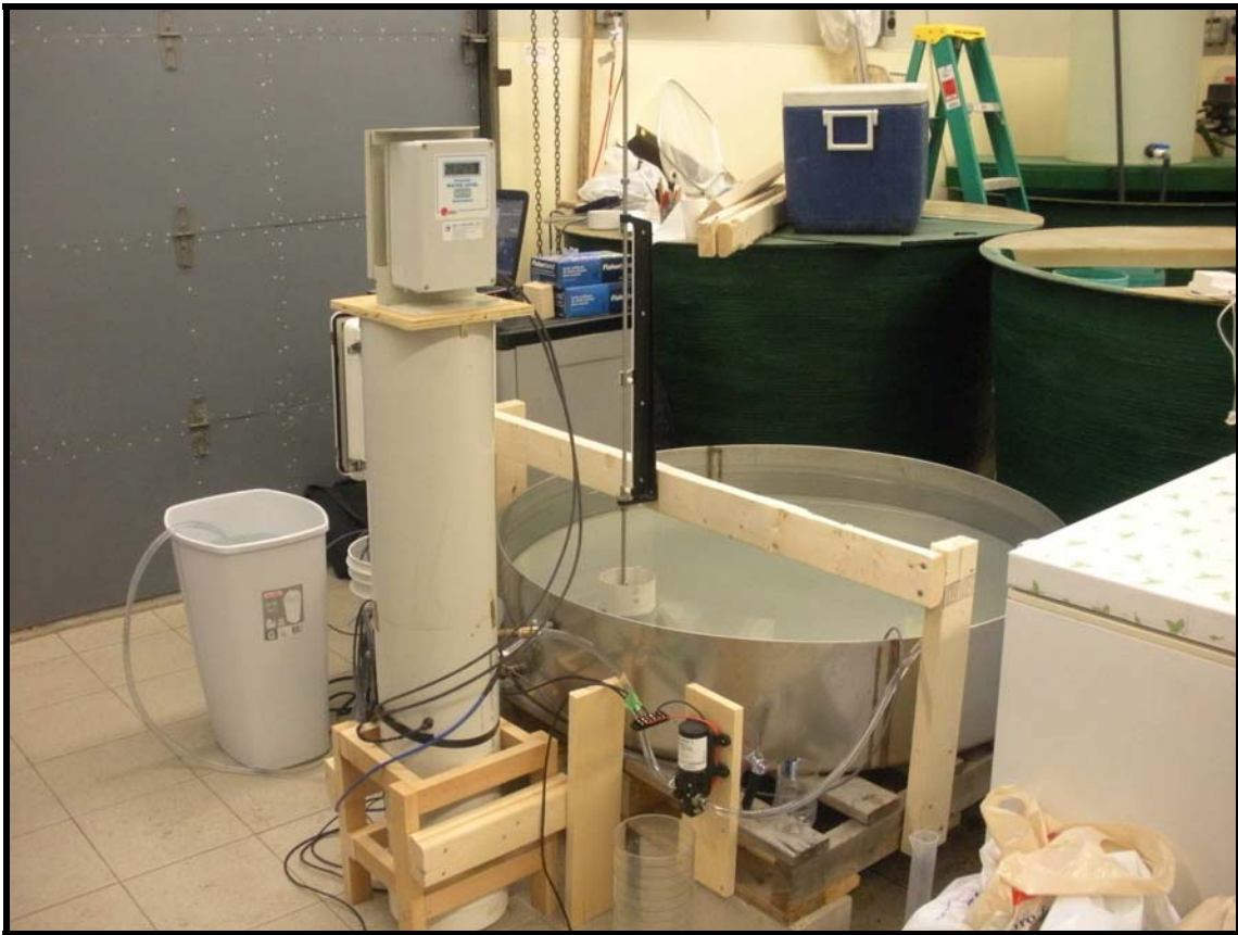
Figure 4. Prototype of the Automatic Evaporation Pan in the lab for testing.
