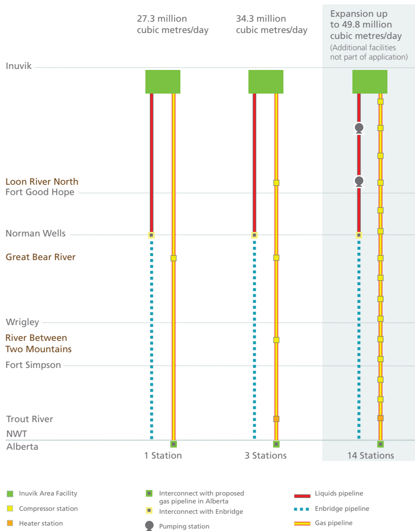
Mackenzie Valley Pipeline design capacity
