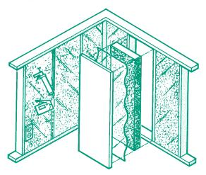
Figure 1. Polyethylene Air Barrier
