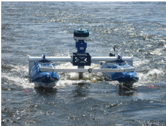
Figure 4 New Energy Corporation: Deployed 5kW EnCurrent Power Generation System
