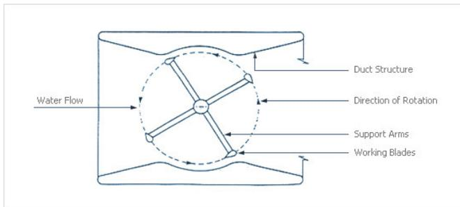
**Figure 2 Blue Energy International Turbine Overhead View**
