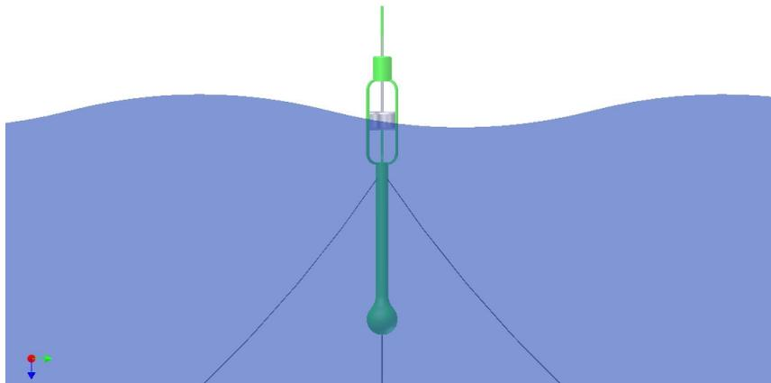
Figure 9 The Sea Wave Energy Extraction Device (SEAWEED™)
