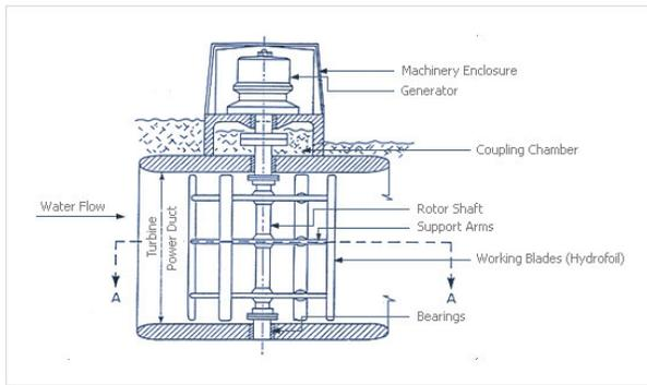
**Figure 1 Blue Energy International Turbine Cross Sectional View**
