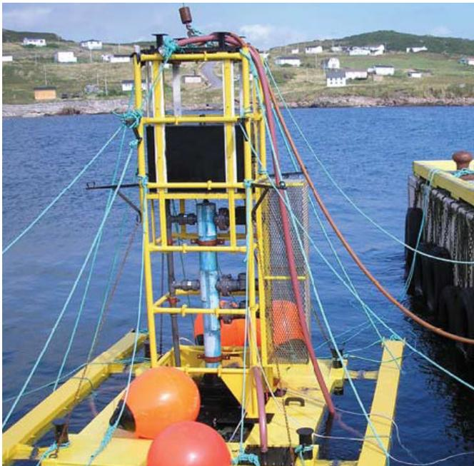
**Figure 8 College of the North Atlantic's Wave-Powered pump**
