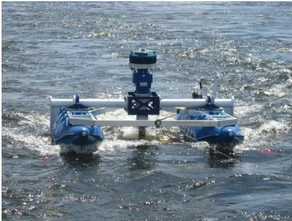
**Figure 4 New Energy Corporation: Deployed 5kW EnCurrent Power Generation System**
