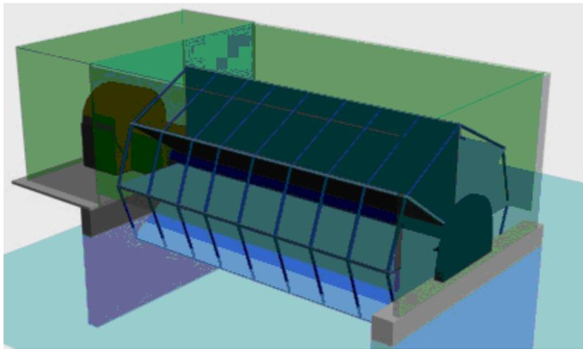
**Figure 7 Conceptual Illustration of Water Wall Turbine**
