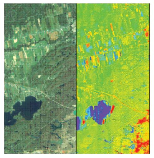
Equivalent water thickness (EWT) is mapped using hyperspectral imagery and by mapping the absorption features of suspended liquid water. Mining activity (south half of the image) is monitored for re-vegetation efforts and mine waste impacts on the surroundings. Agricultural crop vigour is also demonstrated in the north.
