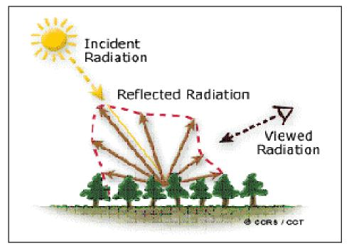
The FLAIR radiative transfer model incorporates wavelength-dependant multiple scattering when simulating interactions between the incident radiation and the vegetation canopy.
