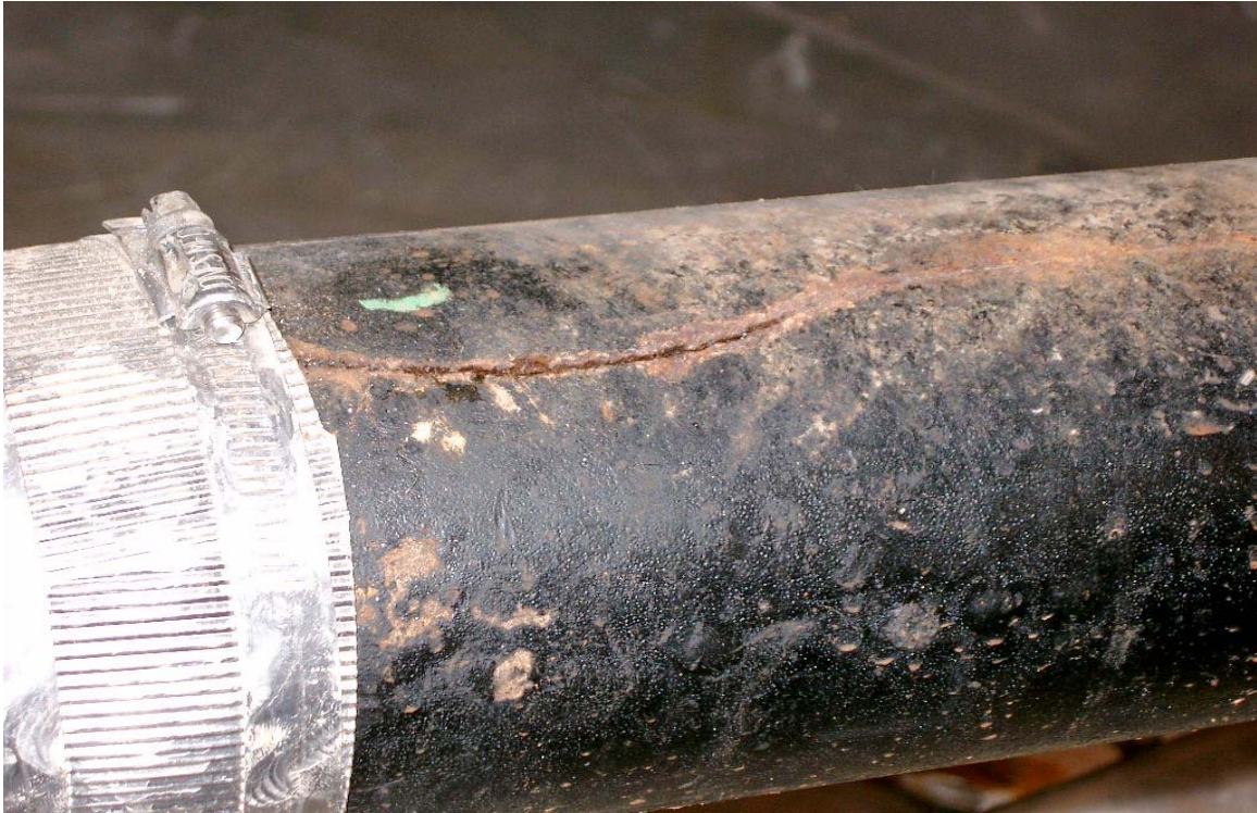
Photo 2: Longitudinal cracks were visible on some piping components. Piping was old, deteriorated and rusty.
