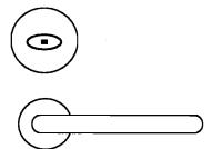
This traditional style of deadbolt has a small, rounded mechanism with a centre pivot point. It is more difficult to grasp and requires greater force to turn.
