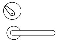
This offset lever deadbolt provides a larger mechanism to grasp, and because it is offset, it requires less force to turn it.
