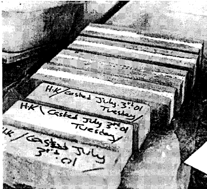
Photo 27: Samples for freeze-thaw tests
