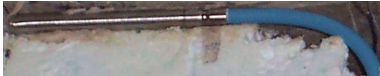
Figure 3: An installed RTD temperature sensor.
