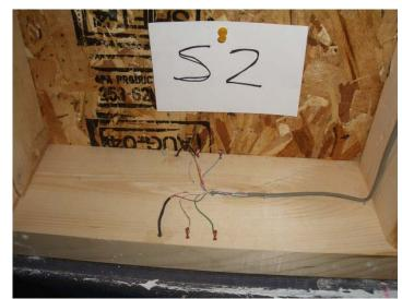
Photo 4.3: No Poly Wall South. No discernable damage or staining visible.
