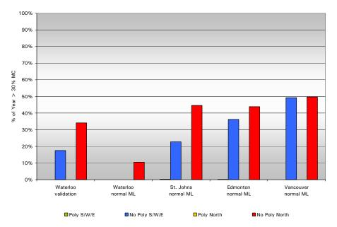
Fig 4.12: Poly/No Poly Walls, Inboard face of OSB, % of Year above 30% MC Threshold
