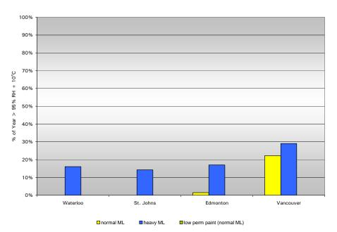
Fig 4.16: XPS North Walls, Inboard face of XPS, % of Year above 95% RH, 10°C Threshold
