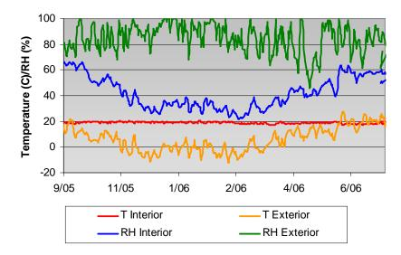
Figure 4.6: Interior and exterior temperature and humidity conditions for basement walls (daily avg. values)
