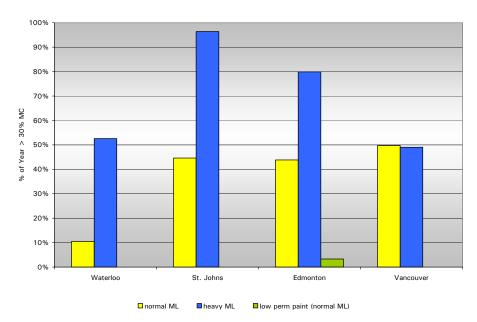
Fig 4.14: No Poly North Walls, Inboard face of OSB, % of Year above 30% MC Threshold
