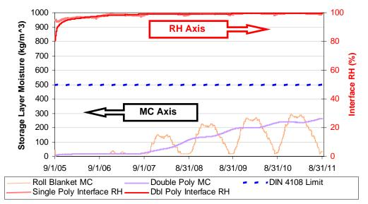
Figure 5.3: Roll blanket and double polyethylene interface condensation layer MC and RH
