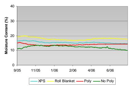
Figure 4.7: Moisture content wafer response, concrete-insulation interface, mid-height (daily avg. values)
