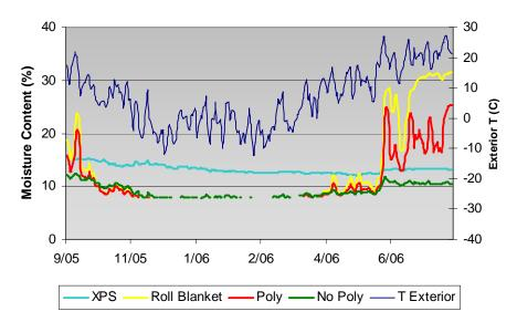
Figure 4.8: Moisture content wafer response, interior side, upper height with exterior temperature (daily avg. values)
