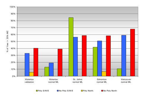
Fig 4.11: Poly/No Poly Walls, Inboard Face of OSB, % of Year above 20% MC Threshold
