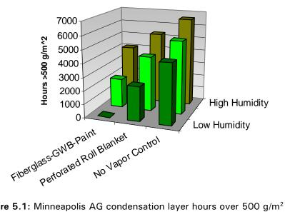
Figure 5.1: Minneapolis AG condensation layer hours over 500 g/m<sup>2</sup>
