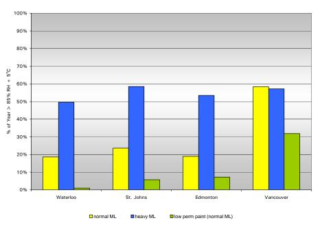
Fig 4.15: XPS North Walls, Inboard face of XPS, % of Year above 85% RH, 5°C Threshold
