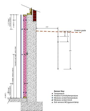
Figure 3.4: Basement exterior monitoring locations
