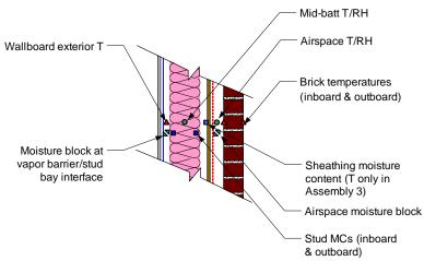
Figure 3.2: Detail of mid-height monitoring locations
