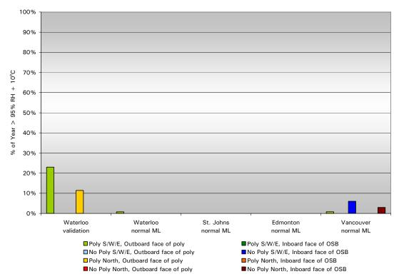
Fig 4.10: Poly/No Poly Walls, % of Year above 95% RH/10°C Threshold
