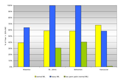
Fig 4.13: No Poly North Walls, Inboard face of OSB, % of Year above 20% MC Threshold
