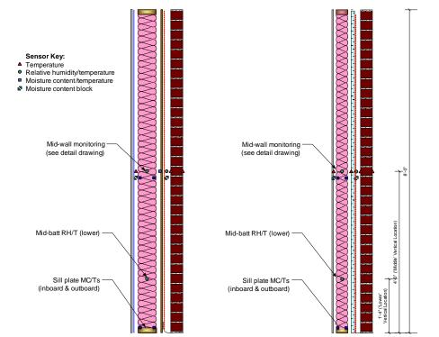
Figure 3.1: Section and monitoring layout for above grade walls 1 and 2 (left) and 3 (right)
