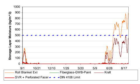
Figure 5.2: Vapour barrier condensation layer MC, Minneapolis above grade, mid RH
