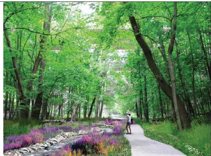
**Prospective:** The trail has been narrowed, surfaced and repositioned alongside the new surface channel which carries the baseflow of Mud Creek. The channel banks are protected by stone interspersed with native vegetative plantings.
