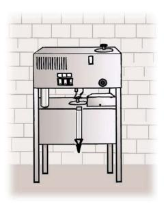
*Energy-saving systems* activate the unit only when a significant amount of water has been withdrawn from the storage tank.
