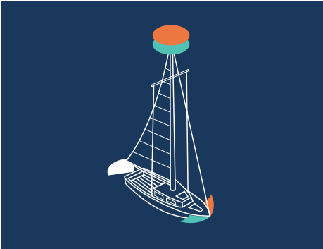
Figure 9-5 Vertical mounted all-round lights
