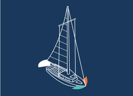
Figure 9-3 Sidelights and sternlight
