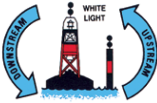
Figure 11-3 Isolated Danger Buoys
