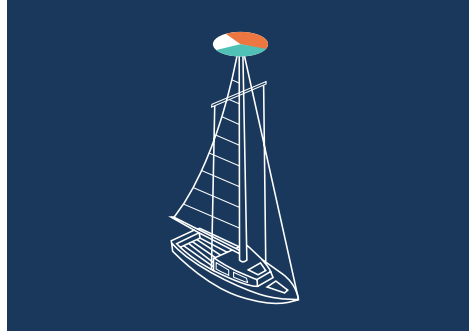
Figure 9-4 Combined sidelight and sternlight
