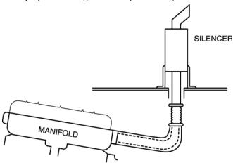
A diverter allowing exhaust gases to pass without restriction *may only* be installed if it is visibly disconnected in a manner that ensures it cannot be easily reconnected while the vessel is in operation.
