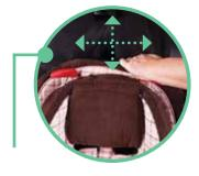
Next, grab the top of the child seat and pull it forward to check the tightness of the tether. It should not move more than 2.5 cm (1 inch) in any direction.
