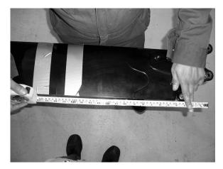
This blade has accumulated approximately 2600 hours, which is about 2/3 of the 3500-hour life limit on this blade. FAA AD 2005-21-02 "Torque Event Inspection" applies to this particular blade.  $\stackrel{\bullet}{\mathbf{X}}$
