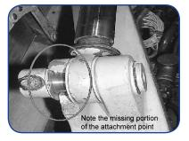
manufacturer Messier Dowty, and the aircraft type certificate holder, Bombardier, are conducting an investigation into this yoke fitting fracture.
