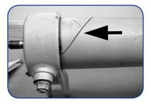
Fortunately, the crack was discovered thus preventing a potentially serious accident and loss of elevator control authority. The type certificate holder has been notified.
