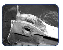
"Z" member, P/N 85311420, on the right side of the wall was also found cracked. Repairs were accomplished in accordance with the manufacturer's instructions.
