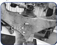
of earlier rework. The crack origin showed evidence of re-work resulting in a non-conforming surface finish and a visible absence of shot peening. Bombardier/ de Havilland has made reference to two earlier investigations on outer cylinder separations. Bombardier/ de Havilland subsequently initiated an information campaign informing fleet operators on the non-recommended practice of single engine taxiing, which produces stress on the NLG assembly.
