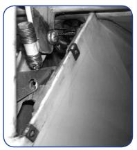
Maintenance personnel removed the elevator bell crank cover and found that the left gusset from the aft stringer support had fallen into the belly of the aircraft. Over a period of time, the gusset worked its way back and became lodged in the narrow clearances around the elevator bell crank.
