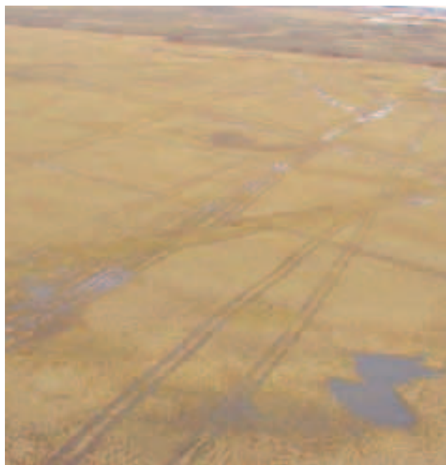
FIGURE 32. (LEFT) Proper use of a seismic line for travel above the treeline. It is apparent that travel was restricted to the planned footprint. (RIGHT) Improper use of a seismic line, showing multiple parallel tracks that significantly increased the project's footprint.
