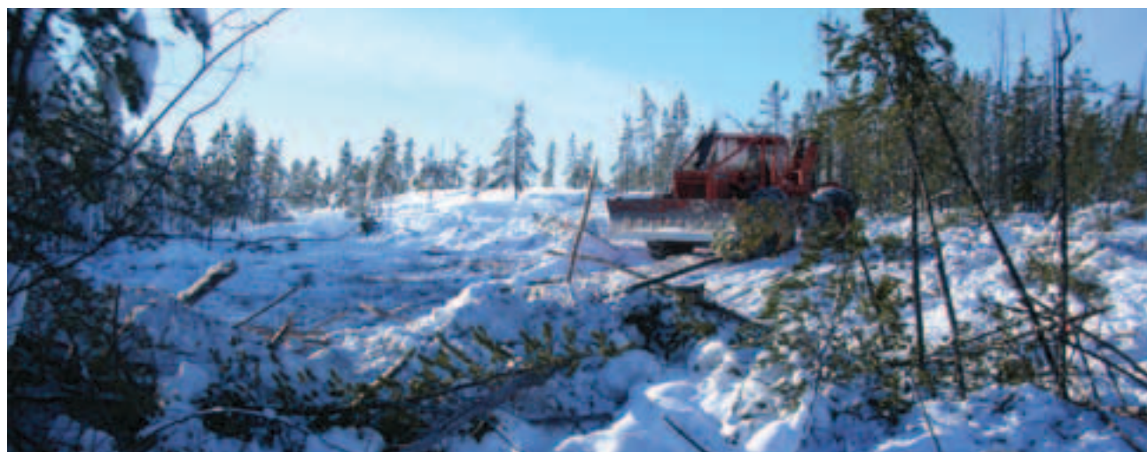
FIGURE 25. Use of a shear blade with a skidder is an acceptable method of clearing in relatively flat terrain.
