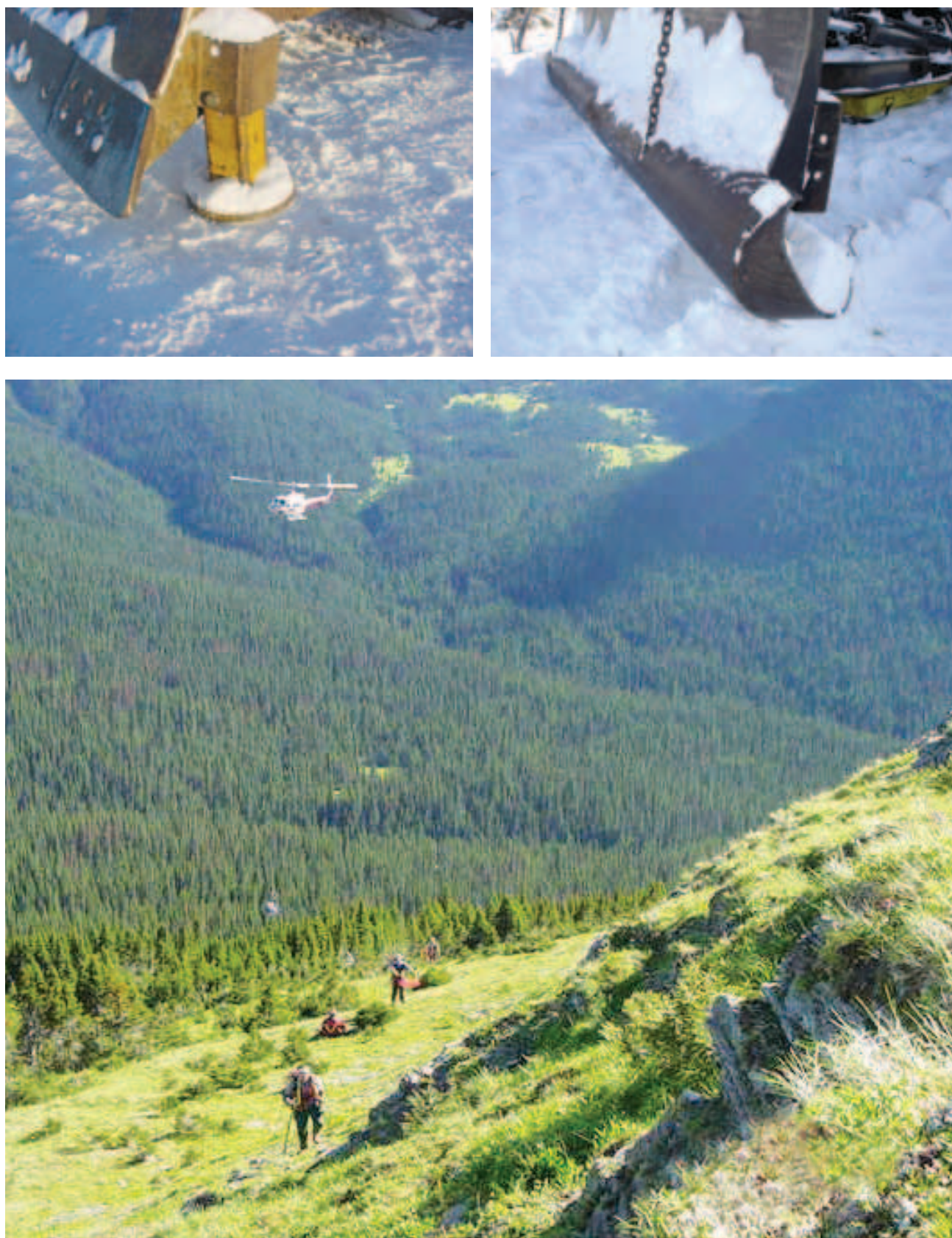
FIGURE 28. (TOP LEFT) Dozer blades equipped with mushroom shoes or (TOP RIGHT) smear blades raise the blade above the ground surface in uneven terrain so that the surface organic layer is less likely to be scuffed or cut. (BOTTOM) Use of heli-portable seismic techniques in steep terrain. Photo courtesy of Explor.
