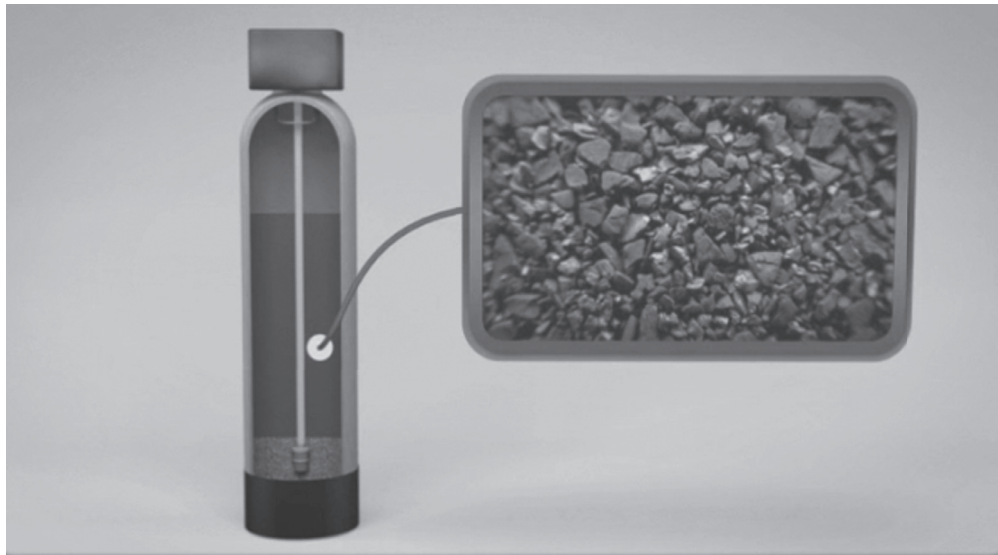
Fig 5.4 A Granular Activated Carbon Filter
