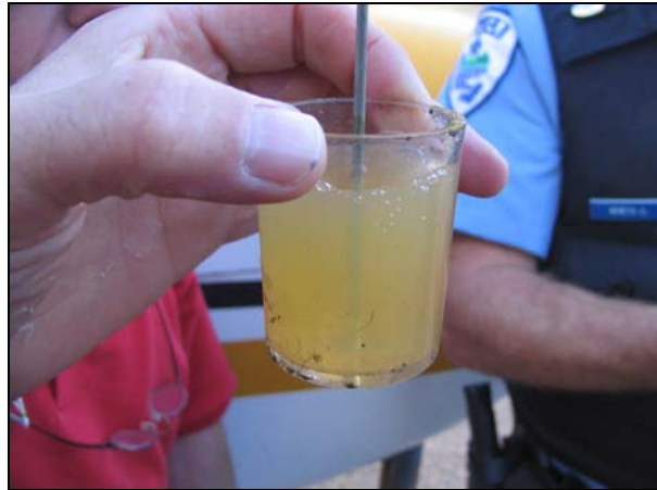
Photo 1. Water from gascolator
