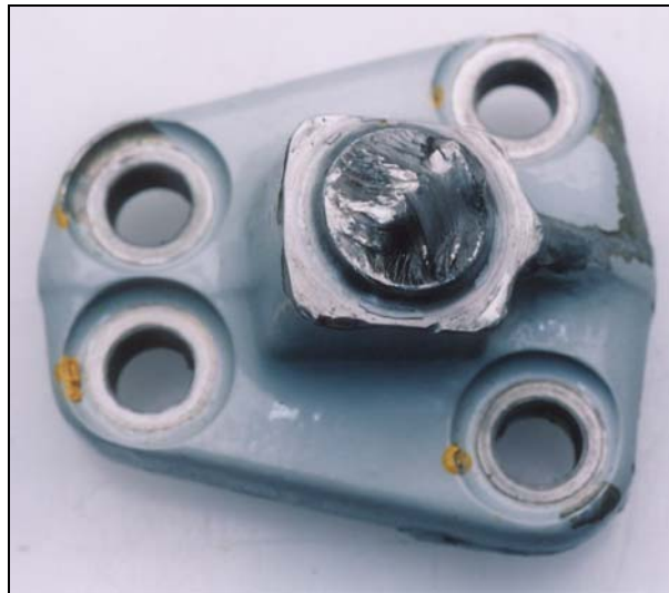
Photo 2. Fractured right-hand pylon support spindle
