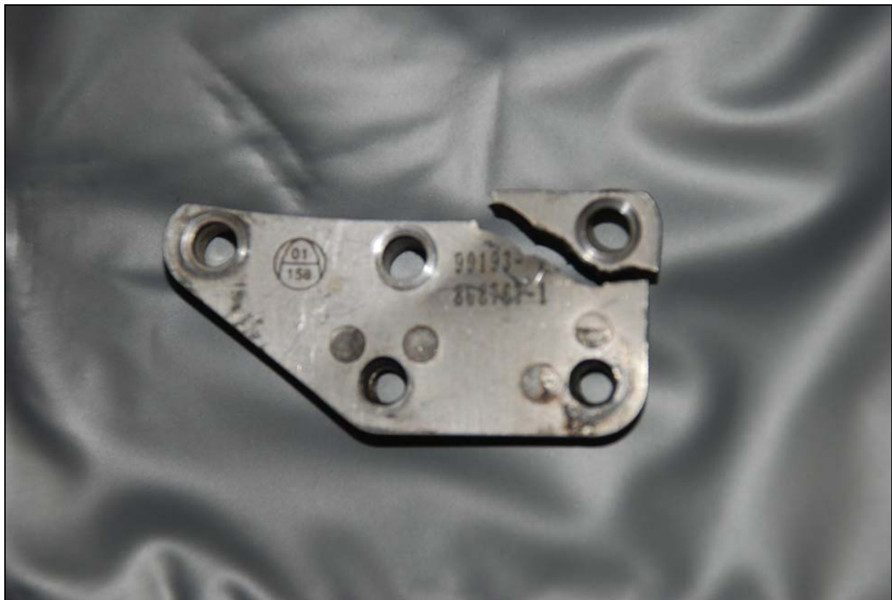
Photo 1. Left engine fuel control upper support assembly
