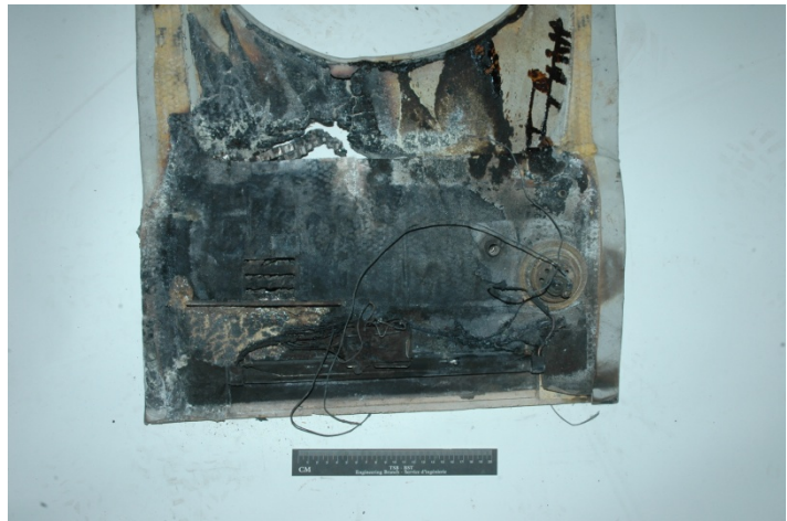
Photo 4. Interior of panel LH/4 indicating where the power supply melted and burned
