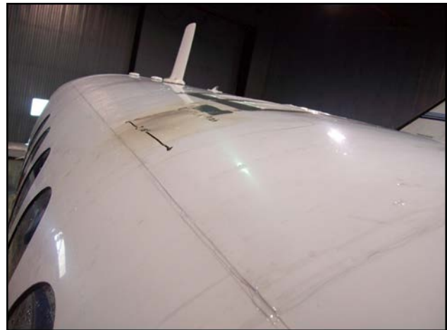
Photo 1. Damage as seen from outside aircraft
